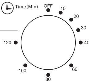
**Timer:** it is possible to set the timer from 0 to 120 min. The furnace will always work before its switch-off manually, at the same time the indicator of operation of the furnace burns.
